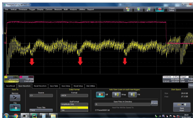
Figure 5: A screenshot from the oscilloscope showing that the instruction pre-fetch leaves a peak on the power trace.
